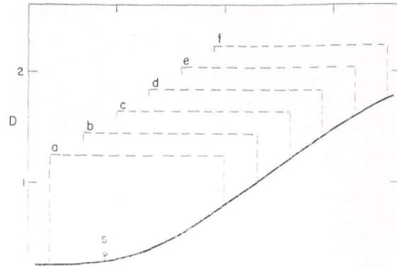
Fig. 4. The  $D$ -log  $E$  curve for the film used in the experimental study of the safety factor. Dashed lines show the log  $E$  positions of the six camera negatives for Scene 1.
