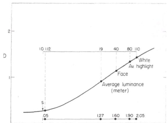
Fig. 9. The exposure levels, for various scene elements, associated with the proposed safety factor of 1.2.
